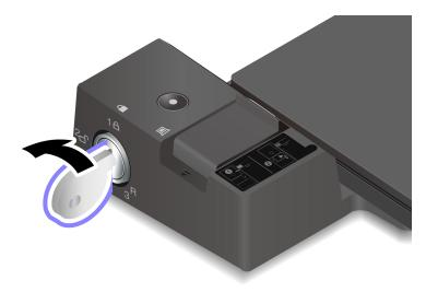
2. Slide the latch in the direction as shown **1** to release the computer, and then grasp both sides of the computer to remove it **2**.
