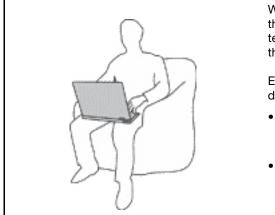
When your computer is turned on or the battery is charging, the base, the palm rest, and some other parts may become hot. The temperature they reach depends on the amount of system activity and the level of charge in the battery.
