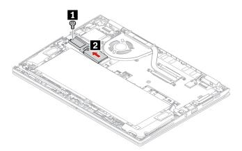
6. Turn over the M.2 solid-state drive with the bracket. Remove the screw **1**, and then separate the M.2 solid-state drive from the bracket **2**.
