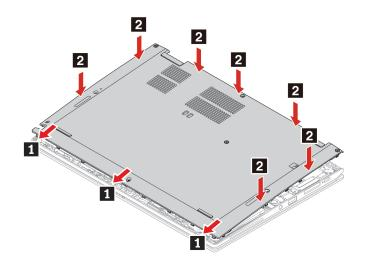
8. Tighten the screws to secure the base cover assembly.
