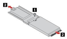
7. Install the new M.2 solid-state drive to the bracket **I** and tighten the screw **2**.
