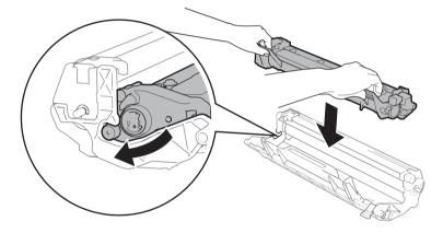
7 Put the drum unit and toner cartridge assembly back into the machine.
