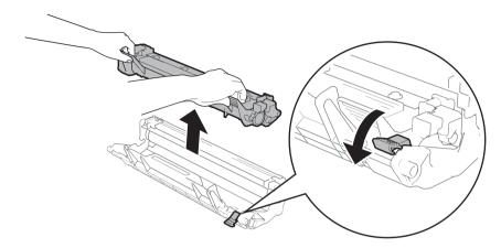
6 Put the toner cartridge back into the drum unit until you hear it lock into place. If you put the cartridge in correctly, the lock lever on the drum unit will lift automatically.
