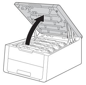
**3** Take out the toner cartridge and drum unit assembly for the color shown on the LCD.
