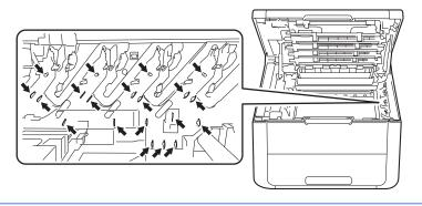
Push down the green lock lever and take the toner cartridge out of the drum unit.
