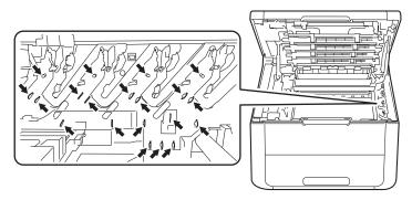
4 Push down the green lock lever and take the toner cartridge out of the drum unit.
