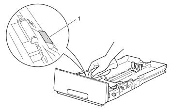
6 Wipe the two pick-up rollers (1) inside of the machine to remove dust.
