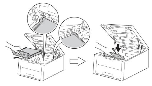
6 Slide each toner cartridge and drum unit assembly into the machine. Make sure that you match the toner cartridge color to the same color label on the machine. Repeat this step for each of the toner cartridge and drum unit assemblies.
