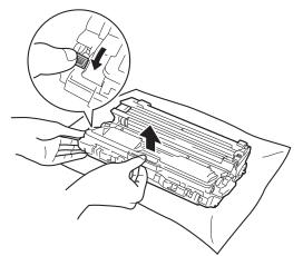
8 Turn the drum unit as shown in the illustration. Make sure that the drum unit gear (1) is on the left side.
