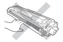
Put the new toner cartridge firmly into the drum unit until you hear it lock into place. If you install it correctly, the green lock lever on the drum unit will lift automatically.
