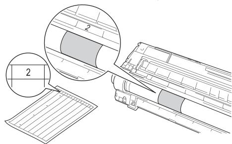
11 Turn the edge of the drum unit toward you by hand while looking at surface of the suspected area.
