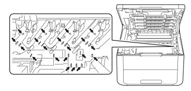
4 Clean the corona wire inside the drum unit by gently sliding the green tab from left to right and right to left several times.
