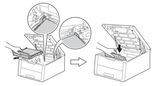
9 Slide each toner cartridge and drum unit assembly into the machine. Make sure that you match the toner cartridge color to the same color label on the machine. Repeat this step for all the toner cartridge and drum unit assemblies.
