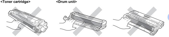
• We recommend that you place the toner cartridge on a clean, flat, level, stable surface with a sheet of disposable paper or cloth underneath it in case you accidentally spill or scatter toner.
