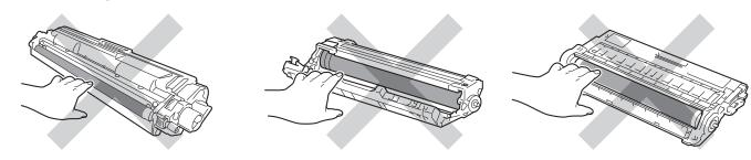
4 Hold the green handle of the belt unit and lift the belt unit up, and then pull it out.
