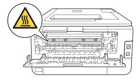
3 Pull the green tabs at the left and right sides toward you to release the fuser cover (1).
