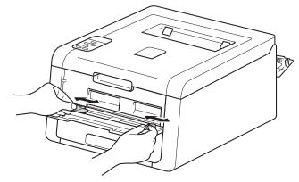
5 Use both hands to push one sheet of paper *firmly* into the manual feed slot until the top edge of the paper presses against the paper feed rollers. Continue pressing the paper against the rollers for about two seconds, or until the machine grabs the paper and pulls it in further.
