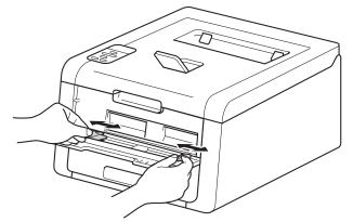
Use both hands to push one sheet of paper *firmly* into the manual feed slot until the top edge of the paper presses against the paper feed rollers. Continue pressing the paper against the rollers for about two seconds, or until the machine grabs the paper and pulls it in further.
