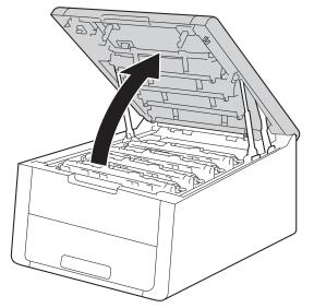
6 The color of printed dots is the color of the drum you should clean. Take out the toner cartridge and drum unit assembly of the color causing the problem.
