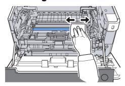
7 On the drum unit, slide the main charger cleaner back and forth 2 or 3 times to clean the charger wire.
