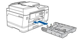
Pull the paper tray completely out of the machine as shown by the arrow.
