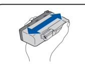
Install the inbox ink cartridges
