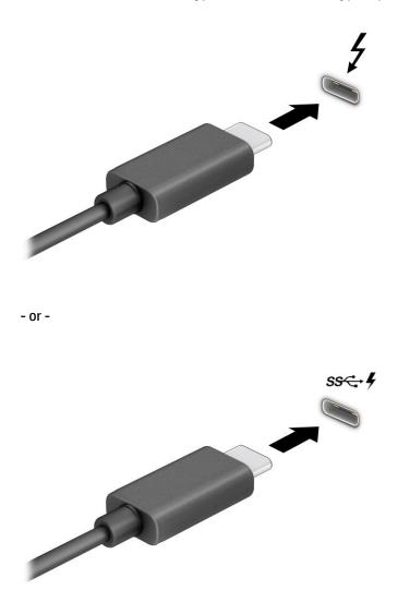
2. Connect the other end of the cable to the external device.
