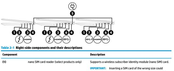
**IMPORTANT:** Inserting a SIM card of the wrong size could damage the SIM card or cause the SIM card to become stuck in the slot. The use of SIM card adapters is not recommended. To prevent damage to the SIM card or the connectors, use minimal force when inserting a SIM card.
