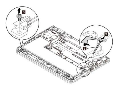
6. Remove the pen charger with the cable from the computer as shown.
