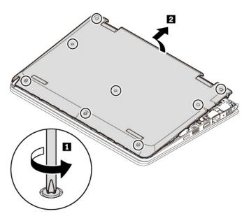
5. Install the new base cover assembly in place. Tighten the screws to secure the base cover assembly.
