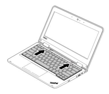
7. Lift the keyboard slightly as shown 1. Pivot the keyboard slightly upward to remove it 1 from the keyboard bezel.
