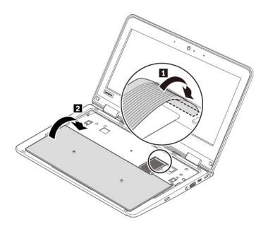
2. Insert the keyboard as shown. Ensure that the front edge of the keyboard (the edge that is close to the display) is under the keyboard bezel.
