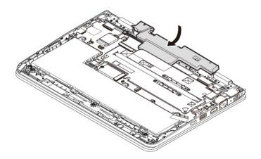
8. Install the screws to secure the speaker assembly **1**. Attach the connector of the new speaker assembly to the system board **2**.
