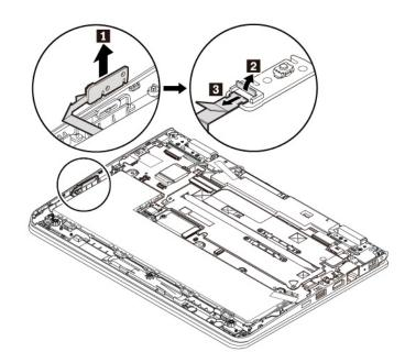
6. Attach the connector to the new power button card **1 2**. Align the notches on the power button card with the notches on the computer. Insert the new power button card as shown **3**.
