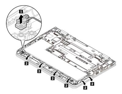
7. Route the pen charger cable as shown **II**. Place the pen charger to the correct location and install the screw to secure the pen charger to the computer **I**.
