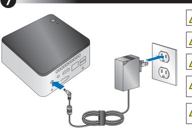
Failure to use the included FSP Group, Inc. Model FSP065-10AABA Power Adapter may violate regulatory compliance requirements and may expose the user to safety hazards.
