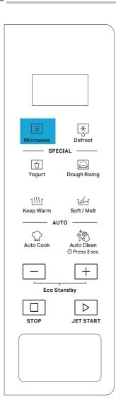
To cook with microwave power individually, press the Microwave button repeatly to select a cooking power level, then press +/- button to set a desired cooking time. The longest cooking time is 90 minutes.
