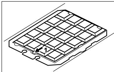
3. To install a new filter, perform the same steps in reverse order. In any case, it is necessary to replace the filters at least every four months.
