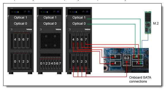
Figure 7. Onboard SATA connections
