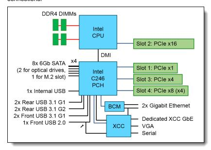
Figure 5. ST250 system architectural block diagram
