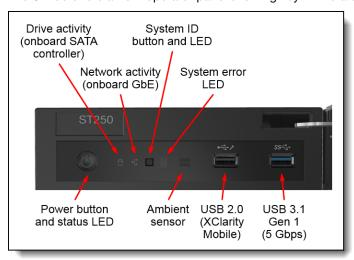
Figure 10. Front operator panel
