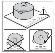
Place the cookware in the centre of the selected zone. Induction cooking zones adapt to the dimension of the bottom of the cookware automatically.
