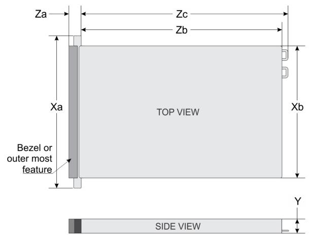
Figure 6. Chassis dimensions
