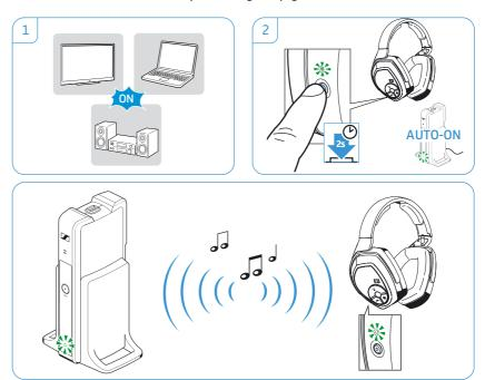
If the headphones are brought outside the transmission range or if there is no audio signal received from the transmitter for more than 5 minutes, the headphones switch off automatically.
