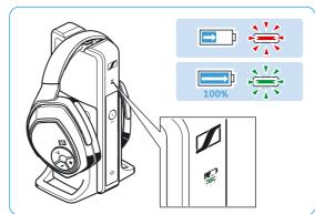
When not in use, place the headphones on the headphones holder to ensure that batteries are fully charged when needed. The transmitter utilizes an intelligent battery charging technology that prevents overcharging.
