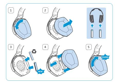
You can also power the headphones using standard batteries (AAA size, 1.5 V). Note however, that standard batteries are not rechargeable, and if you are using non-rechargeable batteries, you must not place the headphones on the headphones holder.
