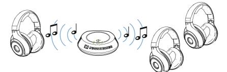
When pressing the transmitter's multi-function button  $\bigcirc$  (1) in multi-user operation, the transmitter switches to single-user operation. You can still listen to your sound source with the last headphones paired, the other headphones are disconnected from the transmitter.
