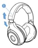
For good sound quality and best possible comfort, the headband has to be adjusted to properly fit your head. To do so, adjust the headband 1 via its snap-in locking mechanism:
