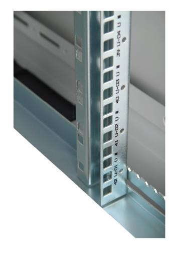
Side Horizontal Support Bar in depth; integrated with 1 set (left/right), 1,5mm thickness Z type made of Steel + 8-12 micron zinc plated side horizontal support bar
