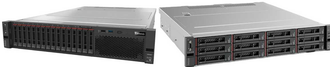
Figure 1. Lenovo ThinkSystem SR590: 16x SFF (left) or 12x LFF (right) drive bays
