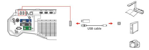
If you connect a digital camera, USB flash drive, or USB storage device, you can use the projector's PC Free feature. You can also connect other Epson document cameras to the projector. See the online *User's Guide* for details.
