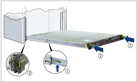
Figure 17: Sliding the server into the rack
