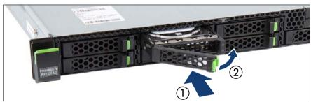
Figure 22: Installing the 2.5-inch HDD/SSD module
