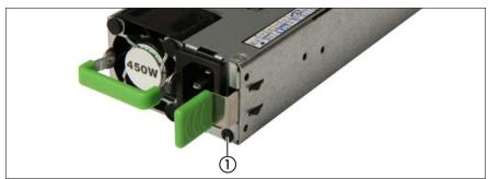
Figure 13: Indicator on hot-plug PSU
