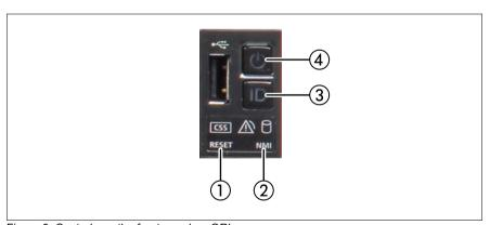
Figure 6: Controls on the front panel on QRL
