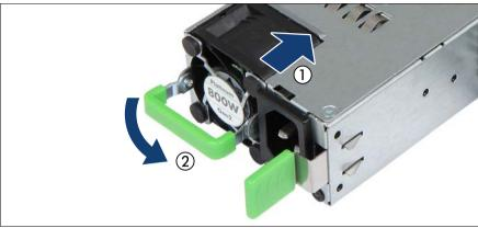
Figure 28: Installing a PSU
