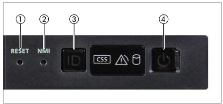
Figure 5: Controls on the front panel module
