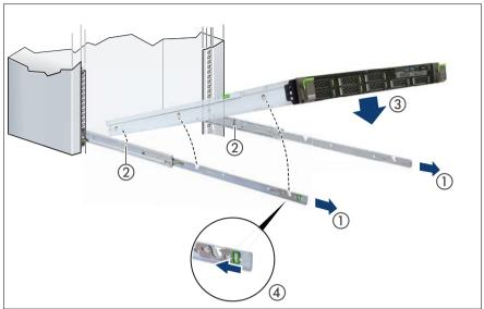
Figure 16: Inserting the server into the rack rails
