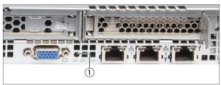
Figure 11: Indicators on the I/O panel: ID, CSS and Global Error indicators
