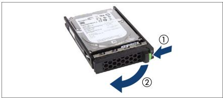
Figure 21: Opening the 2.5-inch HDD/SSD module locking lever
