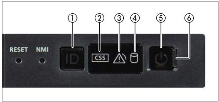
Figure 7: Indicators on the front panel module
