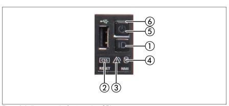
Figure 8: Indicators on the front panel on QRL
