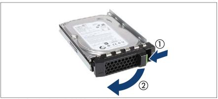
Figure 24: Opening the 3.5-inch HDD module locking lever
