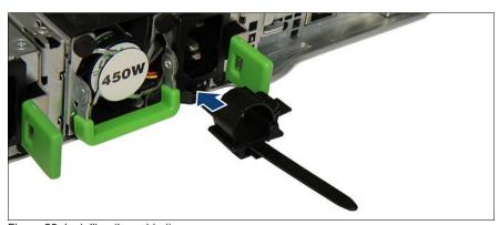
Figure 29: Installing the cable tie
