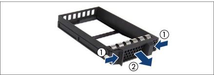
Figure 23: Removing a 3.5-inch dummy module
