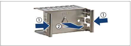
Figure 26: Removing the PSU dummy cover
