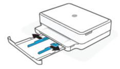
**3.** Insert one or more envelopes into the middle of the paper tray and slide the stack of envelopes in until it stops. The side to be printed on should face down in the printer.
