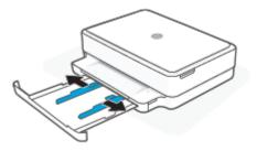
3. Insert a stack of full-size or photo paper into the middle of the paper tray with the short edge oriented towards the printer. For photo paper, make sure the side to be printed on is facing down. Then slide the stack of paper in until it stops.
