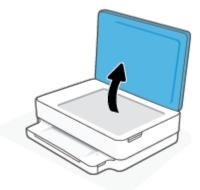
2. Clean the scanner glass and lid backing by using a soft, lint-free cloth that has been sprayed with a mild glass cleaner.
