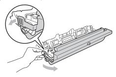
Put the toner cartridge firmly into the new drum unit until you hear it lock into place. If you put the cartridge in correctly, the green lock lever will lift automatically.
