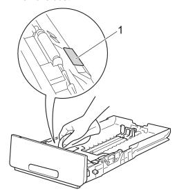
5 Wipe the two pick-up rollers (1) inside the machine to remove dust.
