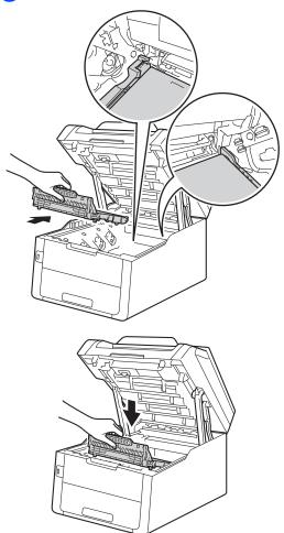
Slide each toner cartridge and drum unit assembly into the machine, making sure you match the toner cartridge colours to the same colour labels on the machine.
