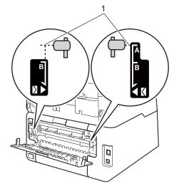
Identify the colour causing the problem and install a new drum unit (see Replacing the drum units on page 82).
