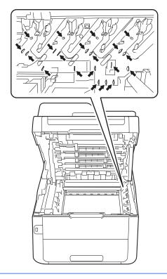
4 Hold the green handle of the belt unit and lift the belt unit up, and then pull it out.
