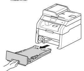
3 Make sure the jammed paper does not remain inside the machine.
