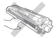
Put the new toner cartridge firmly into the drum unit until you hear it lock into place. If you put it in correctly, the green lock lever on the drum unit will lift automatically.
