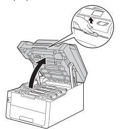
Remove all of the toner cartridge and drum unit assemblies.
