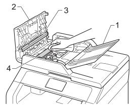
Lift the document cover (1). Clean the white plastic surface (2) and scanner glass (3) underneath it with a soft lint-free cloth slightly moistened with water.
