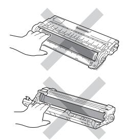
We recommend that you place the toner cartridge on a clean, flat, level, stable surface with disposable paper underneath it in case you accidentally spill or scatter toner. Turn the drum unit as shown in the illustration. Make sure that the drum unit gear (1) is on the left side.
