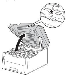
12 The colour of printed dots is the colour of the drum you should clean. Remove the toner cartridge and drum unit assembly of the colour causing the problem.
