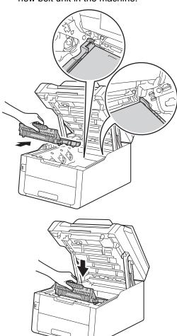
6 Slide each toner cartridge and drum unit assembly into the machine, making sure you match the toner cartridge colours to the same colour labels on the machine.
