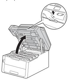
Remove all of the toner cartridge and drum unit assemblies.
