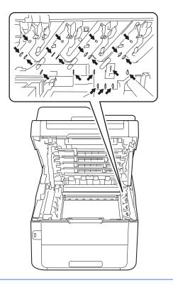
4 Hold the green handle of the belt unit and lift the belt unit up, and then pull it out.
