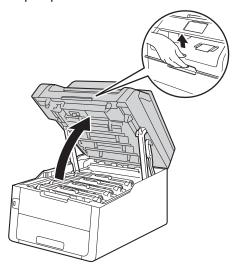
3 Remove the toner cartridge and drum unit assembly for the colour shown on the Touchscreen.
