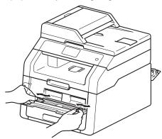
Use both hands to push one sheet of paper or one envelope *firmly* into the manual feed slot until the top edge of the paper presses against the paper feed rollers. Continue pressing the paper against the rollers for about two seconds, or until the machine grabs the paper and pulls it in further.
