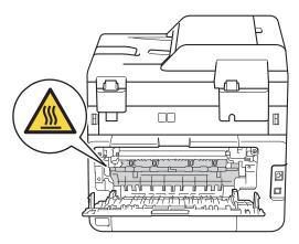
3 Pull the green tabs at the left and right sides down to release the fuser cover (1).
