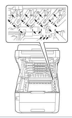
3 Clean the corona wire inside the drum unit by gently sliding the green tab from left to right and right to left several times.
