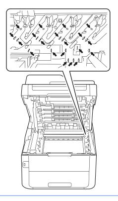
Push down the green lock lever and take the toner cartridge out of the drum unit.
