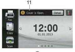
The warning icon ! appears when there is an error or maintenance message; press Detail to view it, and then press to return to Ready mode.
