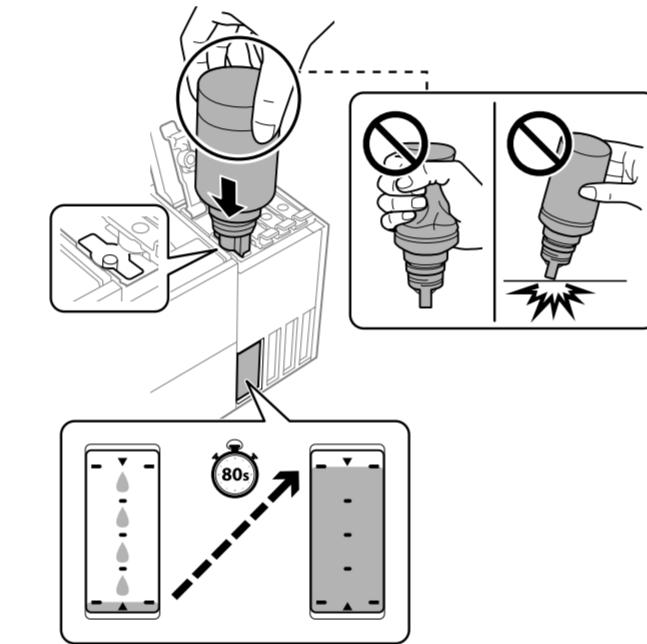
**!** When you insert the ink bottle into the filling port for the correct color, ink starts pouring and the flow stops automatically when the ink reaches the upper line.
