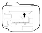
4. Close the cleanout door. Gently push the door towards the printer until both latches snap into place.
