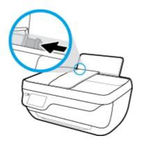
3. Insert a stack of photo paper into the far-right side of the input tray with the short edge down and the print side up, and slide the stack of paper down until it stops.
