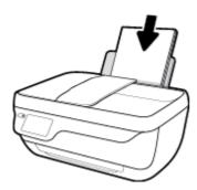
2. Load the original print side up into the document feeder, or load the original print side down on the right front corner of the scanner glass.
