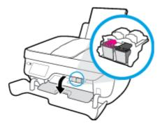
**c.** Press down to release the ink cartridge, and then remove it from the slot.
