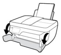
4. Open the cartridge access door and wait for the print carriage to move to the center of the printer.
