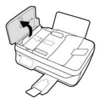
Lift the tab located on the front edge of the document feeder.
